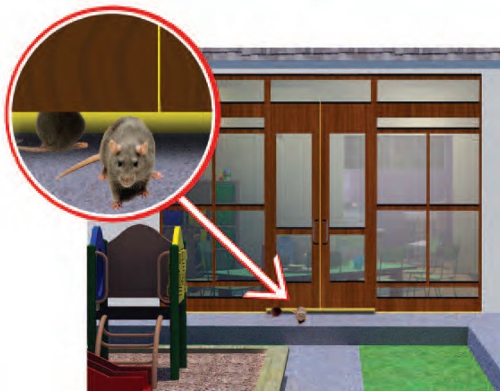
Install door sweeps.
