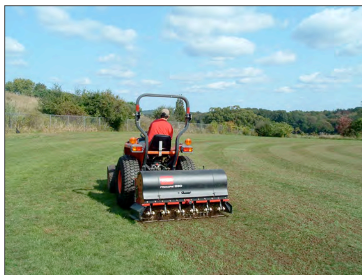
Figure 3. Use only Power Take-Off (PTO) driven, vertically-operating, core cultivation units. These units can provide consistent penetration depth to 3-4". Avoid drum-type core cultivators whenever possible due to their shallow, inconsistent penetration depth.
