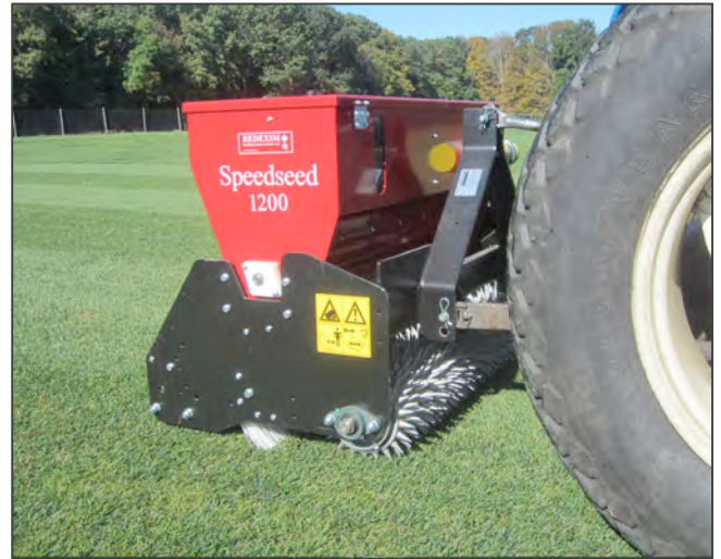
Figure 7. In the absence of imminent cleated traffic, seed should be applied using a spike seeder that will maximize seed to soil contact while minimizing damage to the existing turfgrass stand.
