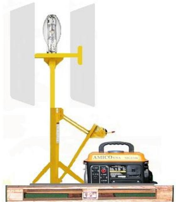
We knew the trap needed to be portable, capable of elevating above the trees tops, and affordable, so this is what I came up with. The trap fits on a skid and can be strapped to a utility vehicle, pick up truck, or can be staked to the ground.
