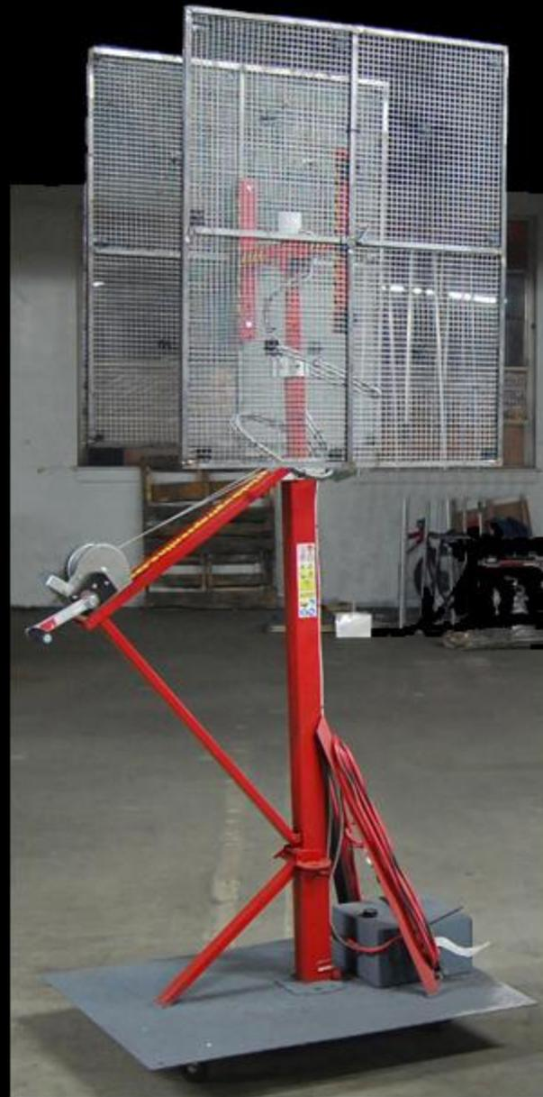
This trap works by electrocution, and it will fry any insect that comes in contact with the electrifying panels. It has been tested and performs just as well as the sticky trap.
