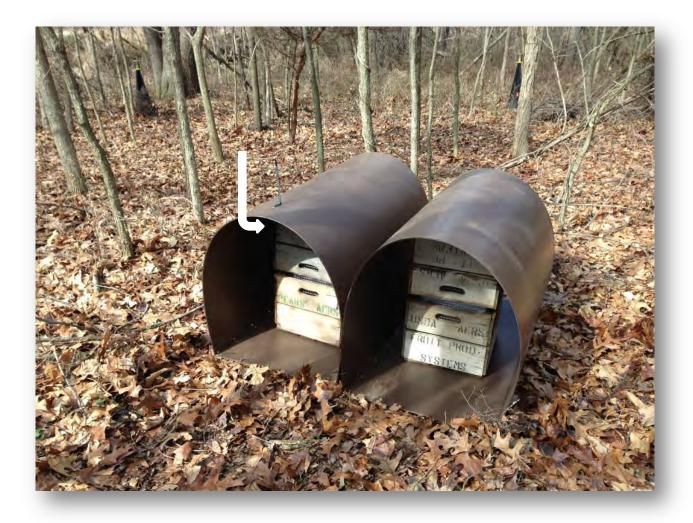
• Temperature/humidity sensors placed inside one shelter and suspended beneath one plastic dome
